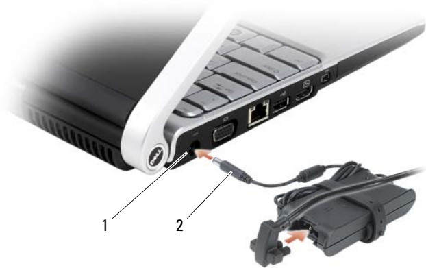
1 AC adapter port 2 AC adapter connector
